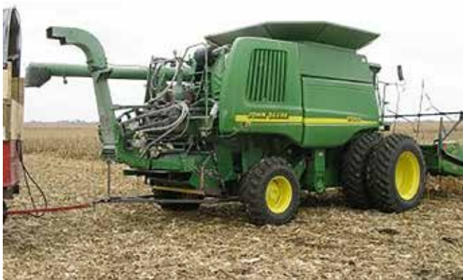
Figure 27: Adaption of the combine: chopper and nozzle (Green Car Congres, 2006)
