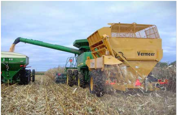
Figure 31: Collection cart with separation of cob and husks (Vermeer, 2009)
