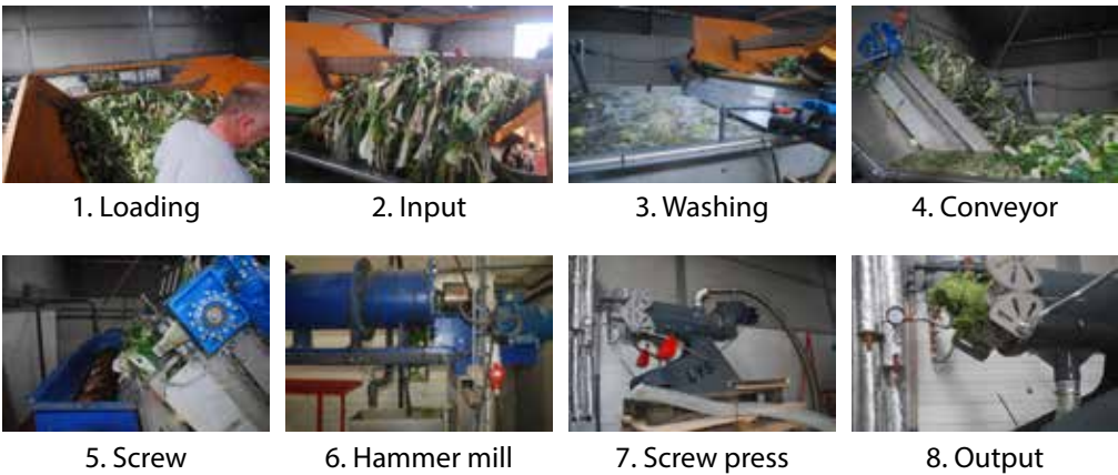
Figure 47: Washing, chopping & pressing experiment with leek residues
