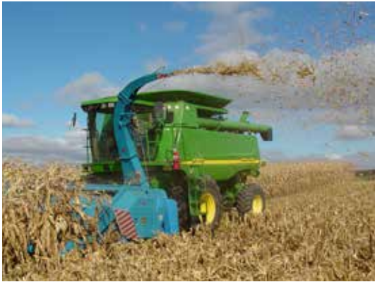
Figure 30: Adapted combine with cutter head to collect and chop stem and leaves (Shinners et al. , 2009)
