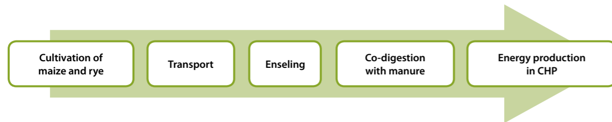
Figure 21: Chart flow of the energy production systems analysed in scenarios 1 and 2
