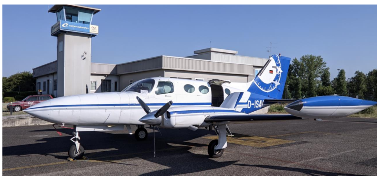
Survey aircraft: twin engine, open camera hatch
