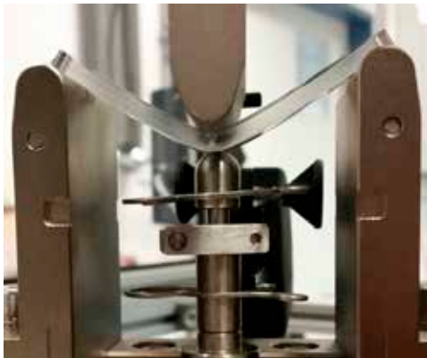
◀ Flexural test on polymer
