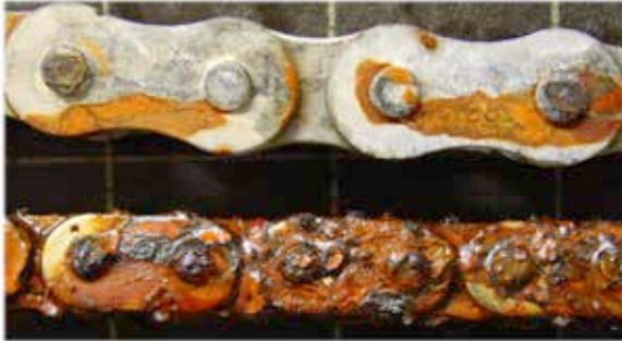
◀ Salt spray test on chain
