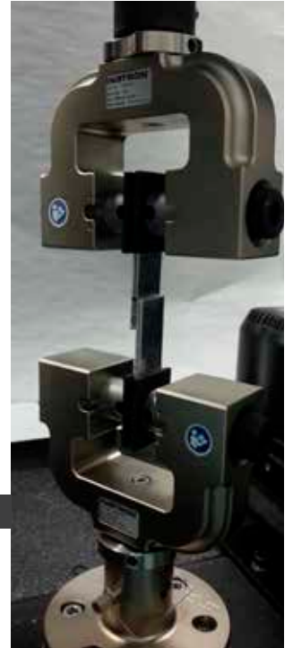
▶ Shear test on adhesive
